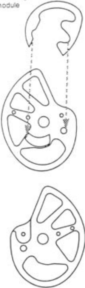
HatchetCams are equipped with modular draw length adjustment. Draw length changes are made by simply changing modules; a bow press may be needed in certain instances. Accessory modules are available from your dealer in one-inch draw length increments. Each module is numbered, with #H1 being the longest draw length module and #H5 being the shortest.
